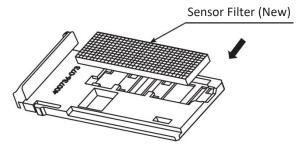
3 After the cartridge is pulled out, remove the old filter as 4 Insert a new filter to the cartridge as shown above and direction shown above.
