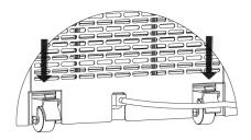
1 Step down the lock lever as shown above 2 Release the rotatable wheels by lifting to secure the rotatable wheels.
