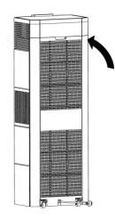
the back cover, turn on the unit and reset the Filter lifespan indicator (Please refer to Filter lifespan indicator reset instruction).
