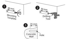
1. Insert the Expansion anchor into the hole (Step 1). Insert the Mounting screw into the Expansion anchor, tighten the Mounting screw by rotating it till it gets fixed steadily and maintain minimum distance of 20 mm (between concrete wall and Mounting screw head) to mount the Water Heater (Step 2). Figure 9
